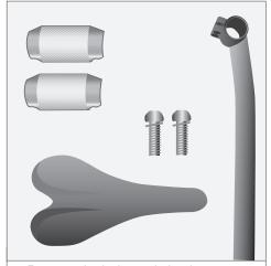
1. Remove the bolts and aluminum carriers from the seatpost.
