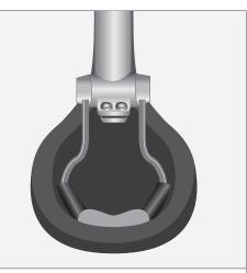
7. Install bolts. Use supplied Ti-Prep. Be careful not to cross thread as the clamp is slightly spread at this point. If needed, squeeze the clamp together with pliers. This is not necessary, but helpful.
