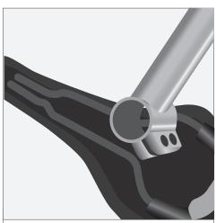
2. Lay the saddle upside down on a table and position the seat post between the saddle rails and insert the upper carrier piece.
