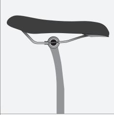
8. Completed Installation. Note the seat post has a slightly set back position.
