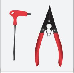
Tools Needed: 5mm Allen wrench, lock ring pliers.
